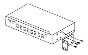
Figure 3. Rack-Mount Kit Side Brackets
